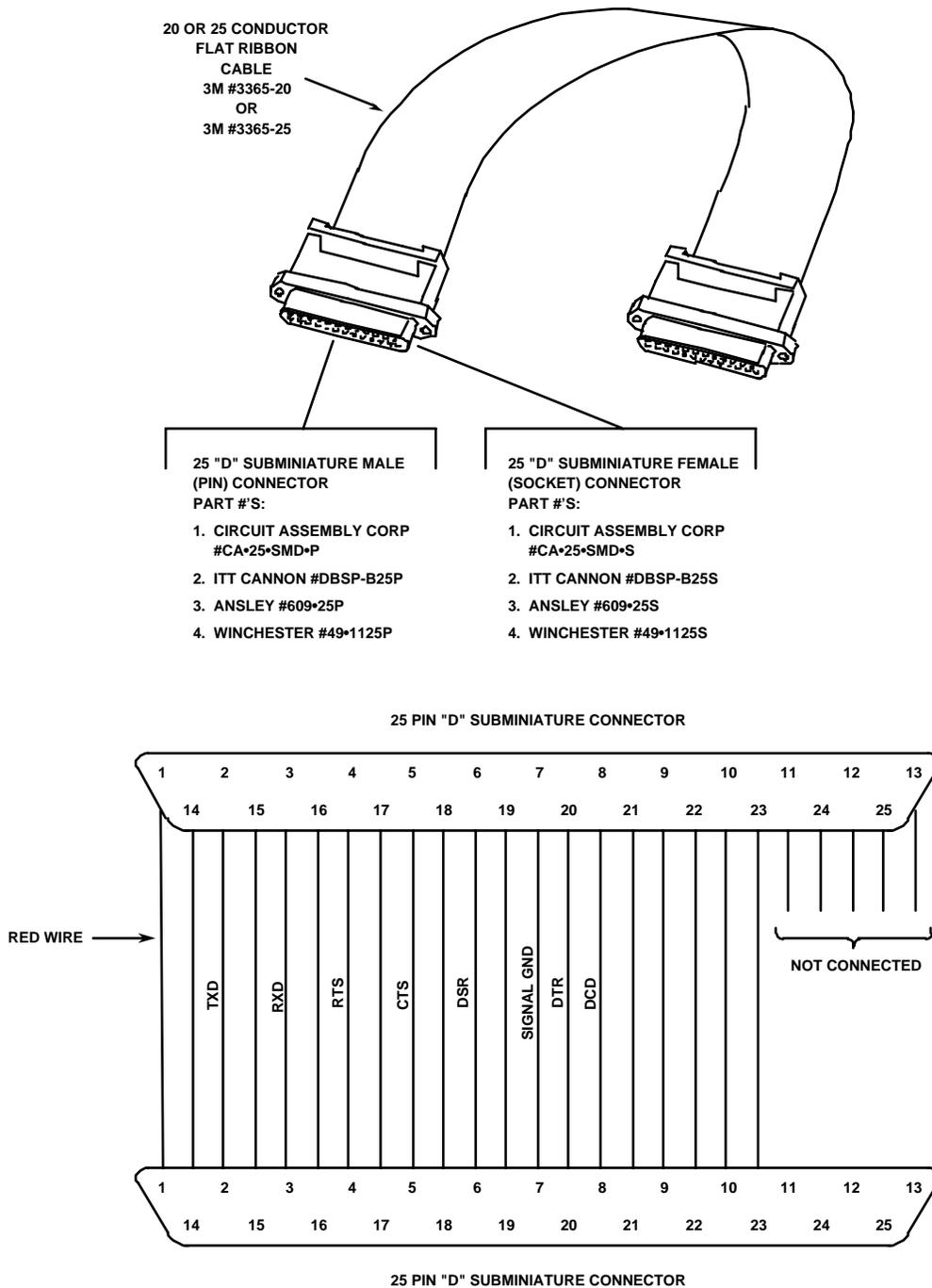
Figure 2-2. Terminal or Host Computer Cable Assembly
