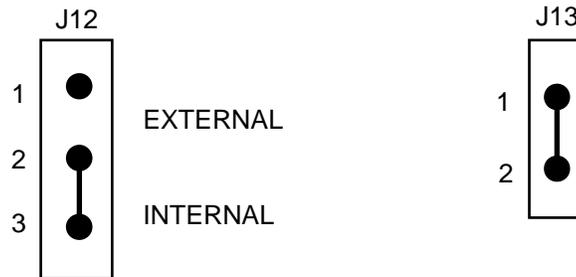
When the external clock source is selected, the user supplies an external clock on the EXTAL' pin (pin 7) of either the SINGLE CHIP connector J1 or the EXPANDED MULTIPLEXED connector J3. If 2 MHz operation is desired, the user must supply an external 8 MHz clock signal via the EXTAL' pin of either connector J1 or J3 (pin 7).
