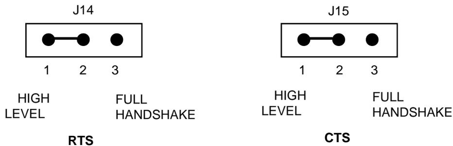
Should the terminal or host computer or modem require full handshake capability, jumpers are to be repositioned between pins 2 and 3. Refer to the schematic diagram located in Chapter 5 (Figure 5-2, sheet 12 of 12) for RTS and CTS signal wiring information.
