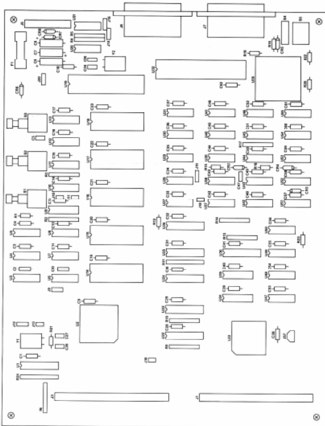
**Figure 5-1. EVM Parts Location Diagram**
